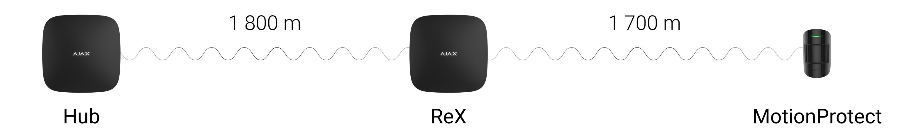
The maximum range of radio communication with connected devices is 1700 meters without obstacles. Up to 5 range extenders can be connected to the Ajax security system. It allows using Ajax products for largescale facilities protection. Regardless of the number of devices connected to the ReX, alarms are delivered in 0.3 seconds.
